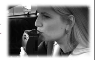
What is it? A breath testing device that connects to a vehicle starter. The vehicle cannot start if the device registers a .02 or more.
